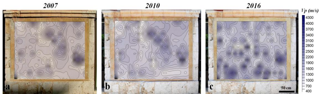
Figure 4: Ultrasonic in time monitoring on an external panel of Sala delle Volte (Exmà): a) ultrasonic survey carried out in 2007; b) ultrasonic survey carried out in 2010; ultrasonic survey carried out in 2016 (after the restoration works of 2014).
